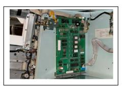
Remove the last hex nut, then carefully lift the door off of the machine. Reverse this procedure to re-install, being very careful when inserting the CPU DIP connector as these 16 pins are VERY fragile and can be damaged easily.
