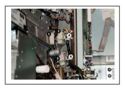
Step 2: Remove ground strap screw C that holds the strap to the upper hinge.
