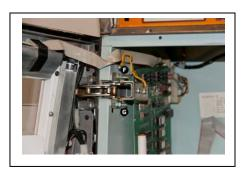
Step 5: Unplug the ribbon cable connector that's attached to the CPU board. Take extra care to be sure you don't damage the fragile pins.
