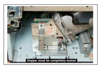
The coin hopper fills up with coins played, and is the "bank" that stores the coins for future payouts. In a casino environment, once the hopper fills completely, a switch on the hopper mechanism senses the weight of the coins and causes any played coins to be diverted to a chute that sends the coins into the cabinet base which the machine sits on.
