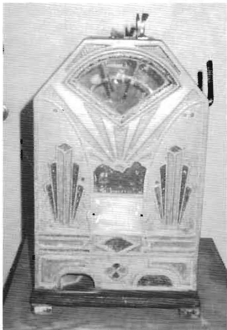
Early LITTLE DUKE production for the export market, summer 1932. The tall Deco arrows are yellow with black middle and red outside wings. Dual payout cup cutouts are evident, a vestigial homage to its French Pierre - Abel Nau parentage, suggesting the color wheel EMPRESS model with small pay out of the left cup and larger pays in tokens on the right. On the LITTLE DUKE only the left cup was used. Play is English Penny, serial 109. Michael Connolly Collection.
