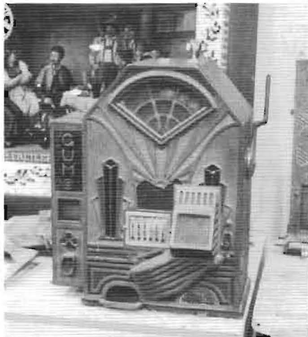
Jennings LITTLE DUKE JACKPOT VENDER MODEL D of October 1932 has plain handle, plain wood right top panel, a jackpot imposed on the front casting and a side gumball vender. The right cup cutout has been used as a patent panel, with copy "U.S.A. Patent No. 1562771 Patent Pending." Deco arrows are black with red and yellow wings. Michael Connolly Collection.
