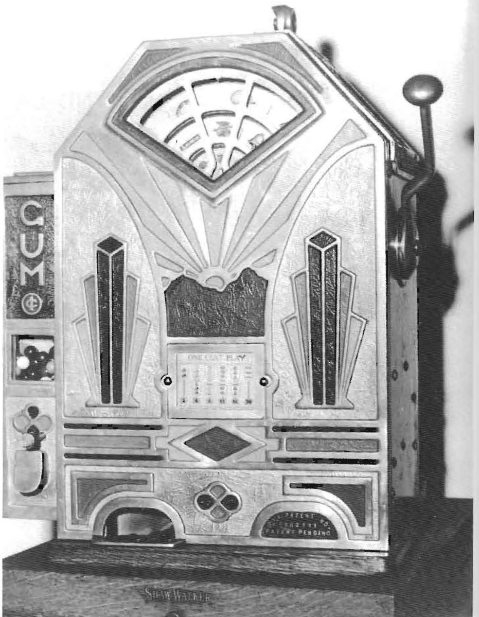
The change is in! The IMPROVED LITTLE DUKE MODEL A of December 1932 has a bullseye coin detector in its top right panel and a knob-headed handle. The 1,562,771 patent number in the lower right panel is for the improved Switch track coinhead which O.D. Jennings filed for patent on December 1, 1924, later to be used on the LITTLE DUKE . Dan Adams Photography.
