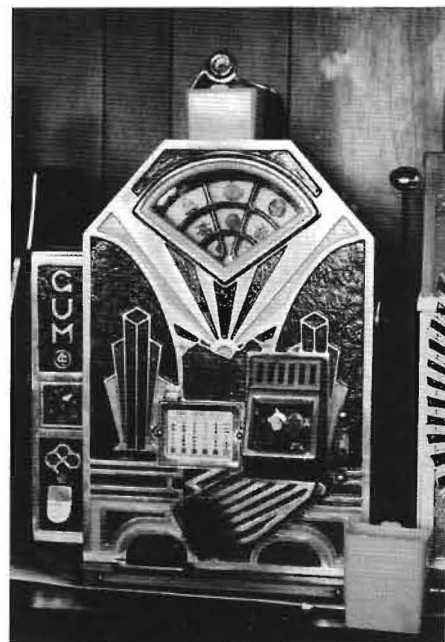
High volume production model of SELECTIVE LITTLE DUKE JACKPOT VENDER in "One Cent Play" has four patent cutout panel, gumball side vender, jackpot knob and selective coin head. Machine serial number is 12,011. Ken Fabian Collection.
